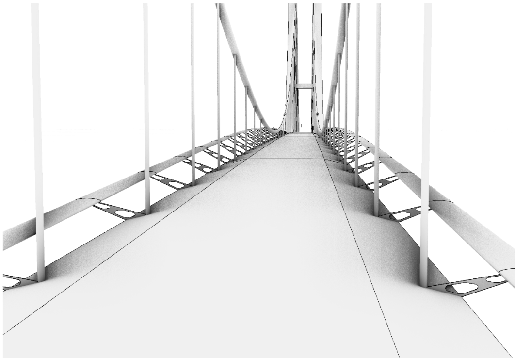
Fig. 6 Bridge with eccentric-wing flutter stabilizer – top view
